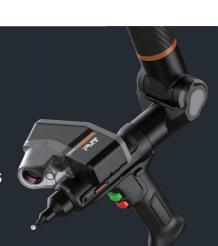
The PMT GAMMA 8-Axis is a complete rotary axis that can be directly connected to the GAMMA ARM. This integration enables a fully enclosed, high-accuracy add-on axis to the portable arm, saving time and effort during hardware setup. Unlike turntables, the 8-Axis is fully transparent to the measurement software and requires no software upgrades.
